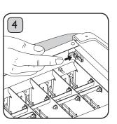
The fuse is reset by depressing the small white button on its face.
