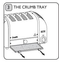
Crumbs will accumulate in the crumb tray and could catch fire if the tray is not emptied frequently. Pull out the crumb tray and wipe clean using a damp cloth. **CRUMB TRAY MUST BE IN PLACE**
