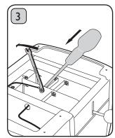
Unscrew brass links and wires.
