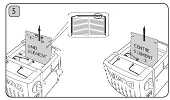
Remove element. To reassemble, reverse procedure ensuring wires and parts are correctly positioned. Ensure new element is marked the same as the one removed. The element heats on both sides and can be inserted facing either way. Check it is seated correctly in the channels either side. Portable Appliance Tested before use.
