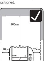
Ensure the Toaster is positioned at least 20cm CLEAR FROM ANY OVERHANGING CUPBOARDS.
