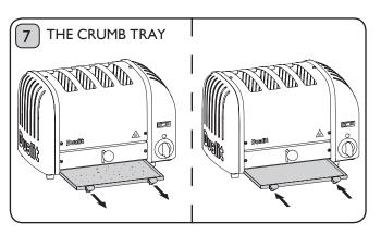
Crumbs will accumulate in the crumb tray and could catch fire if the tray is not emptied frequently. Pull out the crumb tray and wipe clean using a damp cloth. **CRUMB TRAY MUST BE IN PLACE BEFORE TURNING ON THE**
