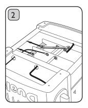
Loosen locking nuts on retaining plate using a 6.5mm spanner and slide back. Ensure that the retaining plate is correctly in position when reassembling.
