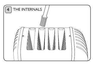
With the toaster unplugged from the power supply use a **SOFT BRUSH** to clean inside your toaster, do not use a sharp or metal utensil! Crumbs should be carefully brushed off the elements using only a soft brush, the toaster can be turned upside down and excess crumbs be shaken out.
