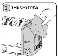
Wipe the aluminium end castings with a damp cloth. Do not use a chemical or abrasive cleaner.
