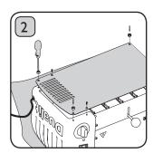
Remove the crumb tray and toaster base plate to access the fuse.
