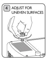
The adjustable foot located on the base of the toaster may be raised or lowered to compensate for uneven surfaces. Rotate it to adjust the height.
