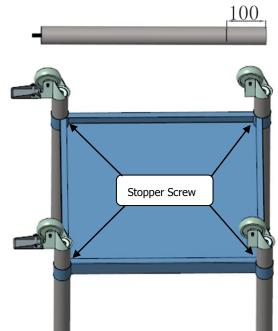
Step 4 - Fix and tighten the screws.
