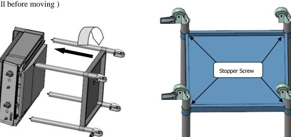
Step 5 – Locate the stand into required position, and adjust the adjustable feet into a level position.
