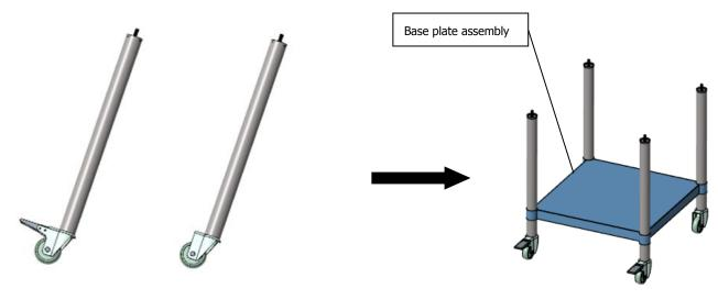
Step 3 –Disconnect, up-turn and support your gas equipment, taking care as items may be heavy. Screw the stand support assembly and castors stand assembly into the gas equipment. ( Remove the cast iron to reduce the weight of the chargrill before moving)
