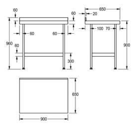
Midi wall tables will align with the Midi range of catering sinks. Midi wall tables are manufactured from 1.2 thick austenitic grade stainless steel polished to a satin finish. Stainless steel underframes complete with shelf are supplied with each table, in a flat pack form with easy to read assembly instructions. Each leg is fitted with an adjustable foot (-20, +10mm) with a working height of 900mm.
