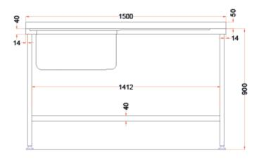
The 1500mm wide flat-packed sink from Holmes is designed with a left side bowl with right side drainer, and is easy to assemble. The sink is manufactured from 304 stainless steel, used for its high resistance to corrosion and physical impact. It is also smooth, hygienic and easy to clean, making it perfect for creating practical and hygienic washing areas in a commercial kitchen. The sink also benefits from a strong undershelf offering additional storage for heavy appliances.
