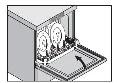
Slide rack into the machine and close the door.
