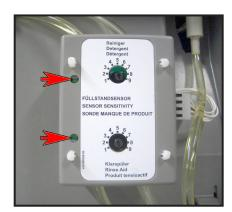
► Observe until the sensor-operated filling of both hoses is complete.
