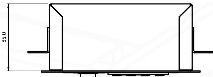
The control box is designed to be fitted on a counter side panel.
