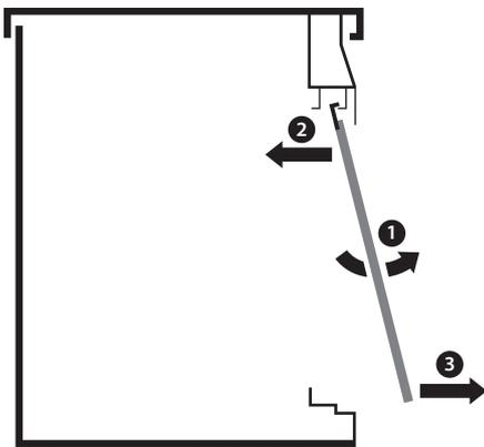
(a) Remove the door bar from the bottom of the doors, by lifting one end up and removing.
