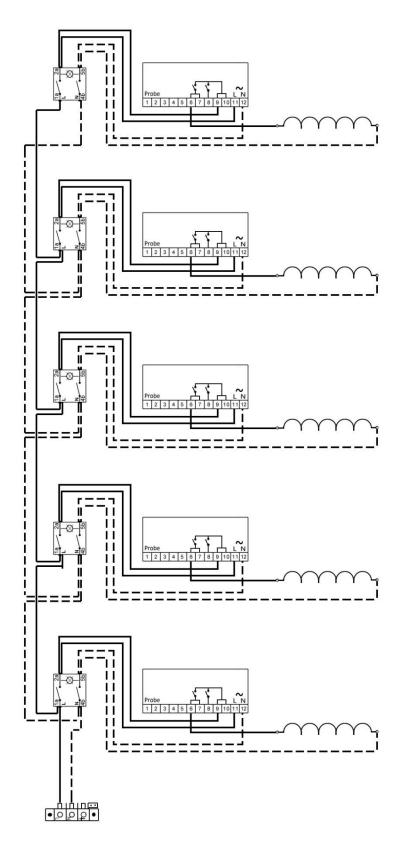
Probe wires are connected to connections 1 & 2 on the controller
