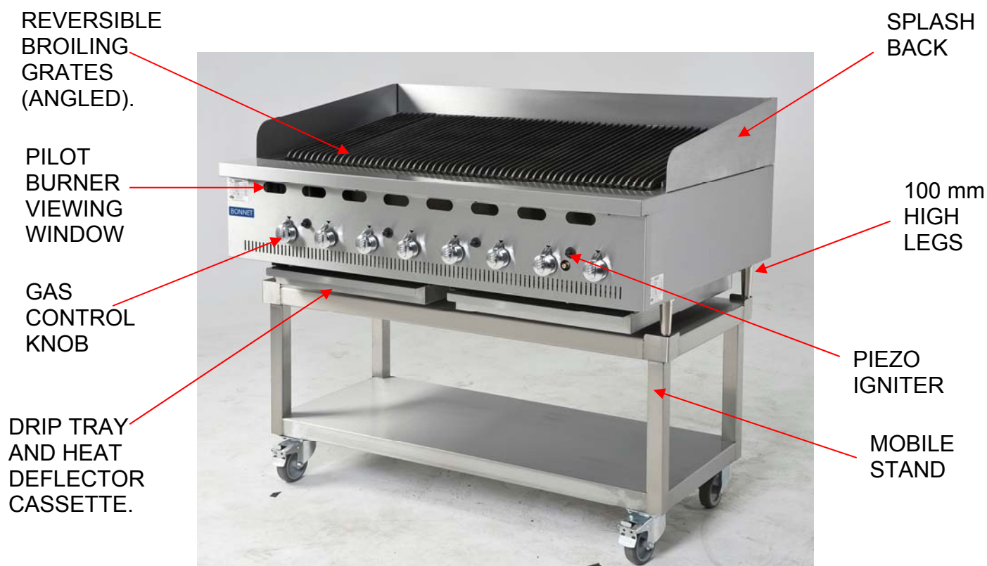
BCB BONNET CHAR BROILER COMPONENT IDENTIFICATION. PHOTOGRAPH 1.
