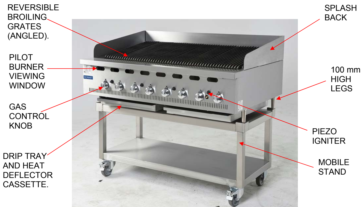
BCB BONNET CHAR BROILER COMPONENT IDENTIFICATION. PHOTOGRAPH 1.
