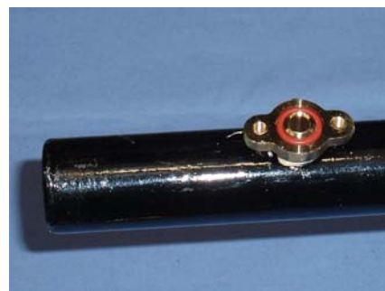
GAS CONTROL VALVE SEAT AND O RING. PHOTOGRAPH 37.
