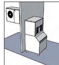
This machine configuration is to be selected for all locations where airflow is restricted, as the refrigerant condenser may be installed remotely vs the ice producing portion of the unit itself, selecting most suitable location for correct condensing temperatures.
