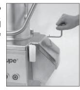
**2** Slide the hinge pin into the slots provided at the back of the motor base.
