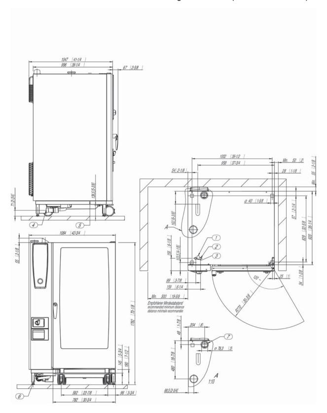
1. Common water supply (cold water) "Single" water connection as shipped 2. Water supply cold water / condensate "Split" water connection 3. Water supply cold / Treated "Split" water connection 4. Water drain 5. Electrical connection wire entrance 6. Chassis Ground connection 7. Steam Vent pipe DN 3" / 78 mm minimum distance 2" / 50 mm Measurements in mm (inch)
