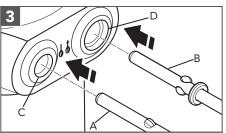
Insert the Beaters without a collar (A) into the smaller opening (C) and Beaters with a collar (B) into the larger opening (D). Align and push to lock into place. Both the Beaters will click in.
