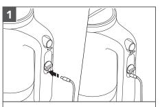
First, slide the Speed Controller to "O" position and insert the Charger Adapter pin into the Charging Port.
