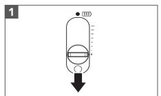
**IMPORTANT:** Make sure that the Speed Controller is at "**O**" position before attaching and removing Beaters.
