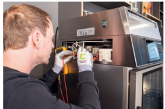
The Convotherm mini's service-friendly design, encountered at every turn, features four service ports and makes servicing and repair easier, faster and more cost effective.
