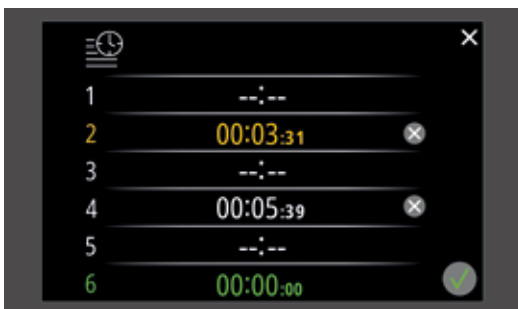
TrayTimer: Indication of the remaining cooking time for each shelf down to the second with color coding.
