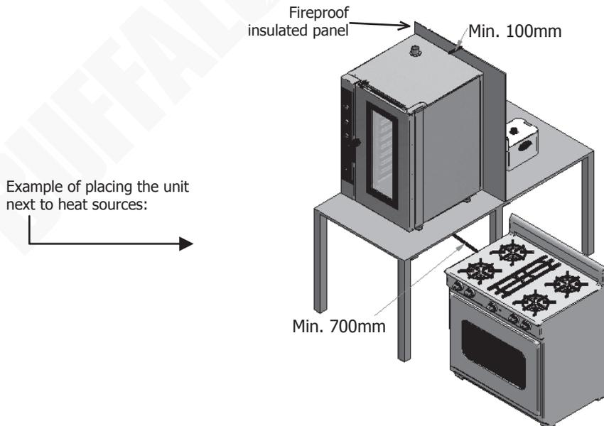
**We recommended leaving a free working space of around 500mm for maintenance operations.**
