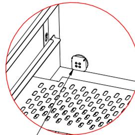
ENSURE THE CAVITY FILTER IS REMOVED AND CLEANED ON A DAILY BASIS, OR AS AND WHEN REQUIRED.
