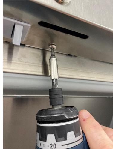
Once this screw has been removed the top panel can be pulled away from the cabinet and slide upwards until the panel is situated on the top of the cabinet. When the top panel is pushed all the way back, it is secured in its position above the cabinet. See the below pictures.
