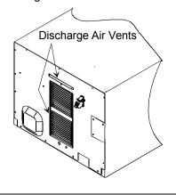
Check monthly for a buildup of cooking vapors along intake and discharge louvers on bottom and back of oven. Clean air vents with damp cloth to ensure proper airflow. Dry thoroughly.
