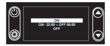
Pressing the up scroll button and the down scroll button for 4 seconds, the data regarding the Filter Time and Water usage are cleaned. If such operation is done in the Status Screen, all the data related to Status are also cleaned (to be used by the service engineer) this feature works only in the Home Screen and Status Screen.
