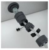
Fit all individual parts onto the cable, as shown in the diagram. Then plug the LAN cable into the port.
