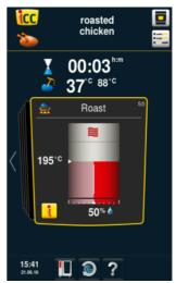
Roast in combination of steam and convection (50% humidity at 202°C cooking chamber temperature).
