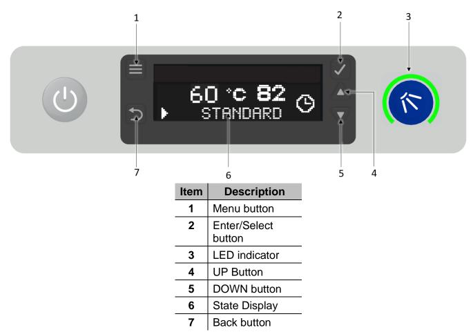
Press Menu button (1) to Enter the Service Mode and Back Button (7) to come out of Service Mode. UP and DOWN buttons (4 & 5) are to scroll the options.
