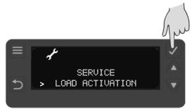
Below is a list of loads that can be activated, via the UP and DOWN buttons (4 & 5), and their required criteria. Each of the loads has a safety timeout applied to reduce the risk of wear on the components.
