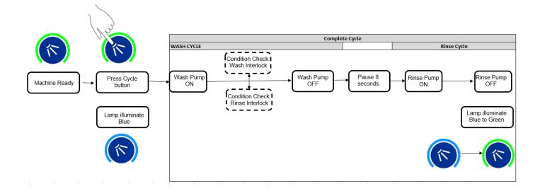
Refer ( $\geq$  7.3.1) for more information on Parameters P41 & P51 and interlock options. Please note if condition for either P41 or P51 not met during specific wash cycle time than it will extend the wash cycle time till it satisfies the conditions.
