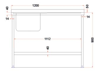
This fully welded 1200mm wide sink from Holmes features a left side bowl with right side drainer, and a strong undershelf providing plenty of extra storage for utensils and cleaning supplies. The sink is manufactured from 304 stainless steel, making it smooth, hygienic and easy to clean whilst highly resistant to corrosion and stains. These properties make the sink ideal for commercial kitchens, allowing you to create practical and hygienic washing areas.
