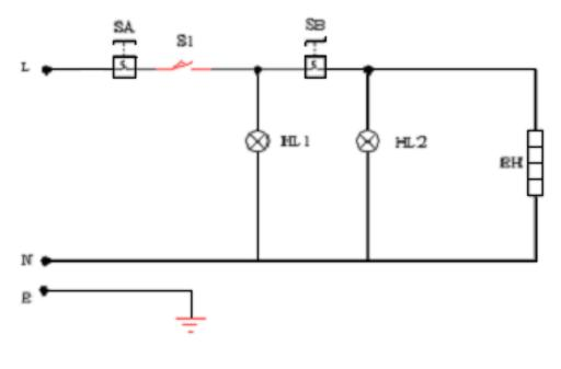
S1—MICRO-SWITCH SB—TEMPERATURE CONTROLLER HL1—POWER INDICATOR E—EARTH OF CASE SA—HEAT BREAKER EH—ELECTRIC HEATING TUBE HL2—HEATING INDICATOR
