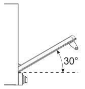
To reassemble the door, put the hinges in the relevant slots in the oven, making sure that grooved sections **C** are resting completely in the slots. Lower the door and once it is in place remove the pins from the holes in the hinges.
