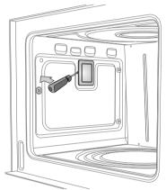
Remove the bulb by unscrewing it as shown. Replace the bulb with one of the same type (25W). Replace the cover correctly, so that the moulded part of the glass is facing the door.
