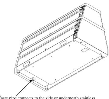
Waste pipe connects to the side or underneath stainless steel Drain Block (3/4" BSPT connection).
