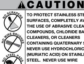
TO PROTECT STAINLESS STEEL SURFACES, COMPLETELY AVOID THE USE OF ABRASIVE CLEANING COMPOUNDS, CHLORIDE BASED **CLEANERS. OR CLEANERS CONTAINING QUATERNARY SALTS. NEVER USE HYDROCHLORIC ACID** (MURIATIC ACID) ON STAINLESS STEEL. NEVER USE WIRE **BRUSHES, METAL SCOURING** PADS OR SCRAPERS.
