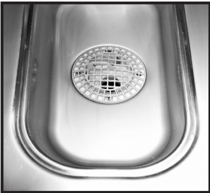
Remove pump intake strainer (rinse section).
