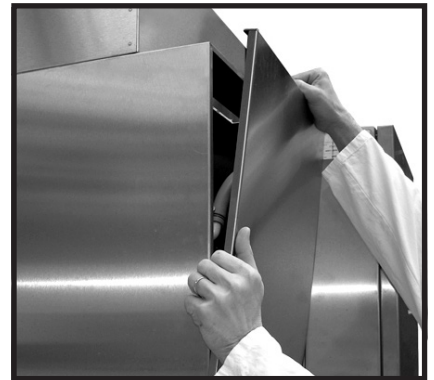
Clean once a month: Remove the front panel of the condenser hood.
