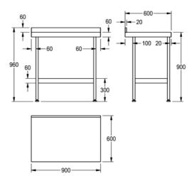
Mini wall tables will align with the Mini range of catering sinks. Mini wall tables are manufactured from 1.2 thick austenitic grade stainless steel polished to a satin finish. Stainless steel underframes complete with shelf are supplied with each table, in a flat pack form with easy to read assembly instructions. Each leg is fitted with an adjustable foot (-20, +10mm) with a working height of 900mm.
