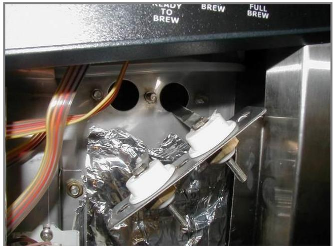
Removal of the Low and High Level Probe assembly
