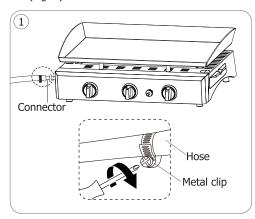
Connect the hose from the griddle to the regulator. Secure the connection with the metal clip on the hose.
