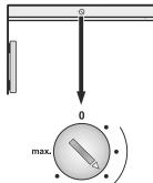
The nearer the temperature control is to the **max.** setting, the colder the interior temperature.
