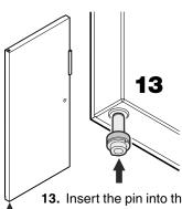
13. Insert the pin into the left-hand door mounting. Use your index finger to hold the pin while you are assembling the door.
