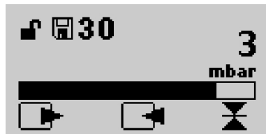
Fig. 13: Sealing status display (050)
