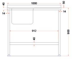
This 1000mm wide flat-packed sink from Holmes is easy to assemble, has a left side bowl and right side drainer, ideal for busy commercial kitchens. The sink is constructed from commercial grade 304 stainless steel, which offers high resistance to corrosion and staining as well as being easy to clean. The sink is ideal for creating practical and hygienic washing areas in your kitchens, and offers extra storage space in the form of a strong undershelf.
