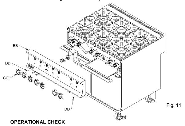
Commissioning must include an operational check of all controls. Check that each burner can be lit at both full rate and low rate. Check that each burner will remain lit when turned to low rate.
