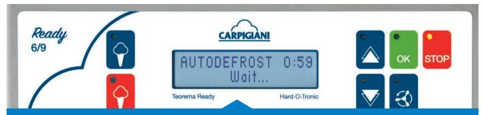
If power is lost during production or the machine is accidentally stopped, an automatic defrost procedure is triggered, allowing for a rapid restart of production.
