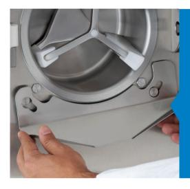
Cleaning is easy thanks to **hot washing** of the cylinder and the removable gelato extraction chute.
