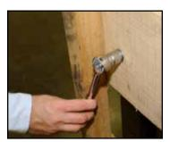
Removing skid from bottom of cabinet.
