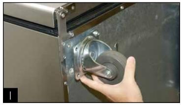
Thread four screws into castor in the underside of cabinet frame rail.
