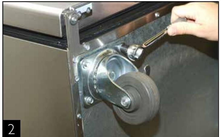
Anchor the four screws firmly to the base of the unit.
