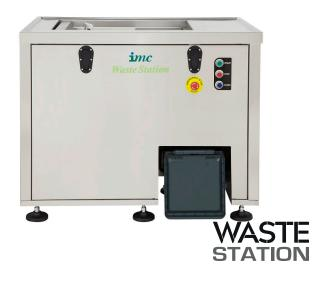
Food waste typically represents around 40% of total commercial catering waste. Of this 40%, approximately 77% is liquid. WasteStation grinds the food waste into fine particles, these particles feed directly into the built-in dewatering system. Through centrifugal action, the WasteStation forces out the excess liquid from the macerated waste.
