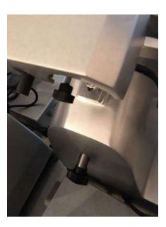
3 Push the bolt upwards once it is completely released. The blade guard is then ready to remove.
