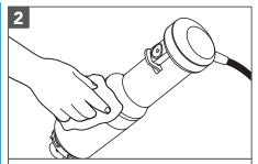
Wipe the Motor Body with a damp cloth. Mild dish soap may be used, but do not use abrasive cleansers.
