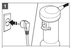
Plug the Hand Blender into an earthed electrical outlet.
