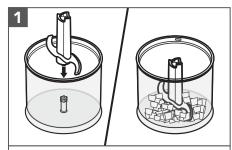
Insert the Chopper blade into Chopper bowl. Add ingredients into the Bowl. For best results, cut the food items into 3/4" (2 cm) pieces.
