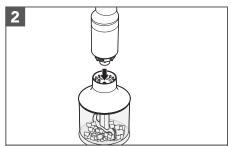
Align the Chopper Attachment with the Motor Body and press together. Do not twist the Motor Body into place.
