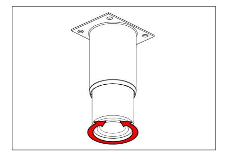
6.4.1 Position appliance and level using feet adjusters as shown below.
