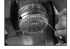
▶ If not, interchange two of the three phase on the feed cable.
