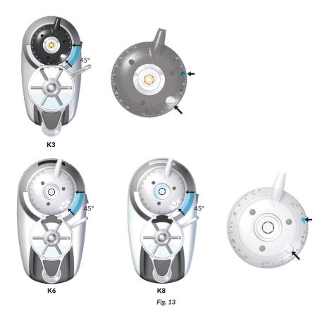
For the models with the micrometric *Parallel* system, first make sure that the grind point lock screw (?) is lined up with the locking foot. This will ensure that the lock screw and locking foot move in conjunction with one another, and that the locking mechanism works properly (*Fig.* 11).
