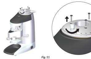
Rotate the grind regulator clockwise until it is completely unscrewed (*Fig. 11*) until the upper and lower burrs touch and can not be turned further. Clean the grind chamber and threads of the housing using a soft cloth and vacuum cleaner until all of the oils and residue has been removed.
