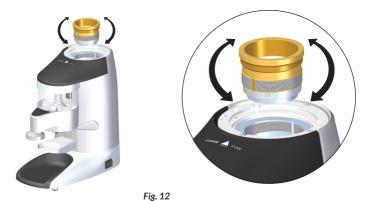
Make sure to put new food grade lubricant on the clean threading of the housing and upper assembly. Insert the upper burr assembly into the grind chamber, and turn counter clockwise.
