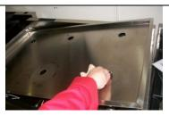
Using an 8mm spanner remove burner injector. Replace with injector from conversion kit. Replace solid top plate, aluminium burner plates and burner caps.
