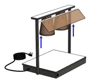
To locate the sneeze guard, align the holes in the sneeze guard with the holes in the underside of the gantry.
