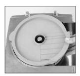
Position the French fries grid in the vegetable preparation bowl. Check that it is correctly positioned with the French fries plate positioned at the outlet.
