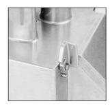
5) Position the head of the vegetable preparation machine on the motorshaft. The fastening hook should now be facing you, on your right.
