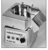
For the R 502 and R 652 models, in cutter version, place the speed selector on the blade drawing in order to operate at 1,500 rpm. For the R 502 V.V. and R 652 V.V. models, the electronic speed variation automatically selects the permitted speed range, which varies between 300 to 3,500 rpm.
