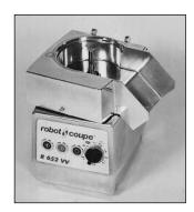
1) With the motor base unit facing your, fit the vegetable cutter bowl onto the motor base unit so that the bowl juts out slightly on the left, with the injection cute on your right.
