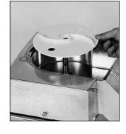
3) Fit the white plastic sling plate onto the motor shaft and check that it is correctly positioned at the bottom of the howl
