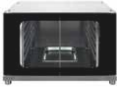
Humidified prover for ovens series ALFA341. Max temperature 60°C, distance between the trays 70mm, 230V 1N 50Hz - 2kW. Dim. (WxDxH) 920x940x600 mm LEV341XV capacity 12 trays
