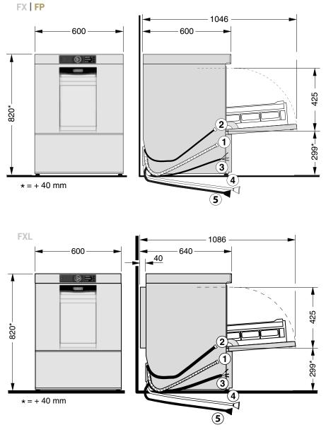
flexible drain hose ② fresh-water connection ③ power cord ④ hose for detergent al ⑤ hose for rinse aid al al for machines with external containers
