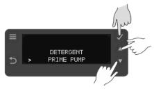
Press Select Button (2) to enter the PUMP operation options. Press UP Button (4) & DOWN Button (5) to select your choice of operation. Confirm your selection by pressing Select Button (2).
