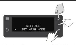
Press Select Button (2) to enter the SET WASH MODE settings Press UP Button (4) & DOWN Button (5) to select wash mode either Glasswasher or Dishwasher. Confirm your selection by pressing Select Button (2).
