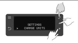
Press Select Button (2) to enter the CHANGE UNITS settings Press UP Button (4) & DOWN Button (5) to select units in either Centigrade C or Fahrenheit F . Confirm your selection by pressing Select Button (2).
