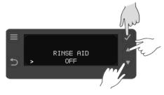
By pressing UP Button (4) & DOWN Button (5), you can set the chemical refill reminder notification ON. Press Select Button (2) to confirm the selection. Default is set to OFF.
