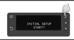
**STEP 3:** Select type of warewasher, Glass or Dish using Up & Down buttons (5 & 6). Confirm the selection by pressing Select button (3).
