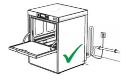
Your warewasher should be placed in a location that allows the electrical, supply water and waste water connections to be fitted ( $\triangleright$ 4.3).
