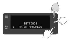
Press Select Button (2) to enter the Water Hardness settings Press UP Button (4) & DOWN Button (5) to select water hardness value. Confirm your selection by pressing Select Button (2). Default is set at highest level 30°DH.
