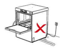
When positioning your warewasher, ensure that the water inlet, chemical tubes and drain hoses are not kinked or squashed. Care must also be taken to ensure the warewasher does not rest on any of its supply hoses / leads.
