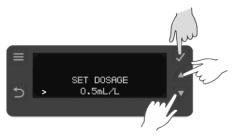
Adjust Rinse Aid dose by using button (4) & (5) as per the concentration required in millilitres per litre of Water (ml/L). Confirm the selection by pressing Select button (2). Default is set at 0.1ml/L.
