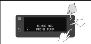
Press Select Button (2) to enter the PUMP operation options. Press UP Button (4) & DOWN Button (5) to select your choice of operation. Confirm your selection by pressing Select Button (2).
