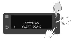
Press Select Button (2) to enter the ALERT SOUND option Press UP Button (4) & DOWN Button (5) to select value. Confirm your selection by pressing Select Button (2). Default is set to OFF.
